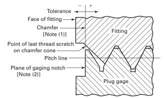
GENERAL NOTE: Enlarged view showing chamfered internal thread of basic size with chamfer exceeding the major diameter.
